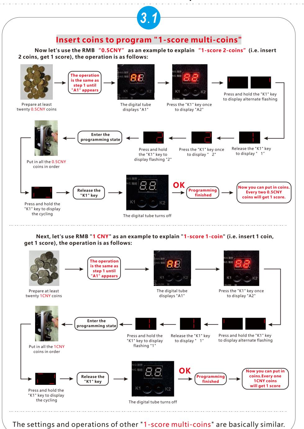
After programming, the coin acceptor saves the signal parameters of "1-score 2-coins" (0.5 CNY) and "1-score 1-coin" (1 CNY), a total of 2 "groups". When using, you can put in two 0.5 CNY coins to get 1 score, or put in one 1 CNY coins to get 1 score. scores can be accumulated.
