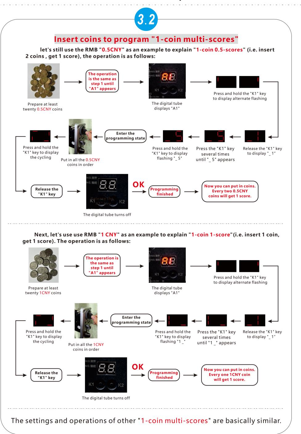
After programming, the coin acceptor saves the signal parameters of "1-coin 0.5-scores" (0.5 CNY) and "1-coin 1-score" (1 CNY), a total of 2 "groups". When using, you can put in two 0.5 CNY coins to get 1 score, or put in one 1 CNY coins to get 1 score. scores can be accumulated.
