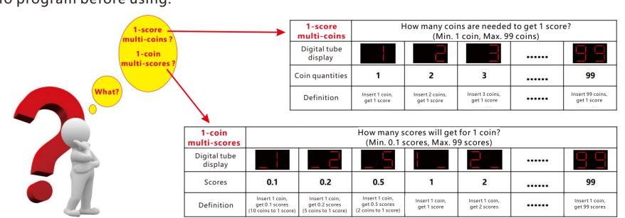
According to the type and denomination of coins, users can program and save the signal parameters of coins by adopting the mode of "1-score multi-coins" and "1-coin multi-scores" respectively. For details, refer to illustration "3.1" or "3.2" below.
